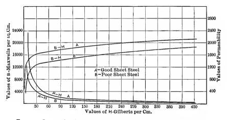
FIG. 32. Curves showing magnetic qualities of good and poor sheet steel.
